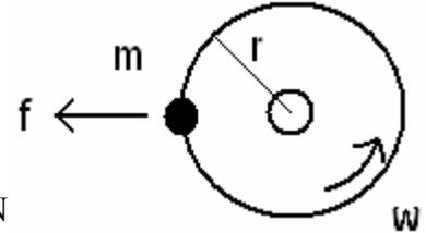
Obviously the imbalanced force is proportional to the mass of the object, and the size, so the proper balancing of large or heavy objects is more important than small, light objects. Also notice that the magnitude of the imbalance force is proportional to the *square* of the speed, so balancing is very critical in high speed applications.
