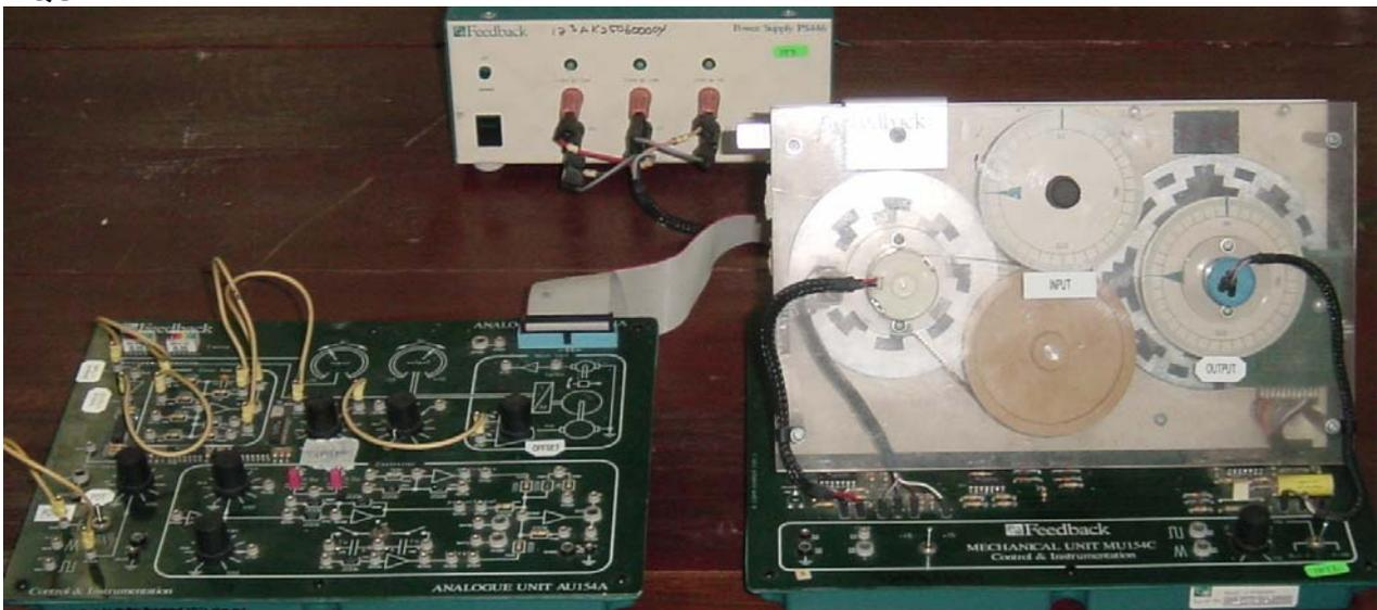
This lab uses the Feedback Instruments Power supply PS446, Mechanical Unit MU154A and Analog Unit AU154A interconnected as described in the “*Servo Fundamentals Trainer*” manual SFT154. In addition you will need a stopwatch.
