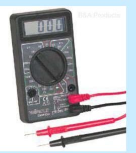
To measure currents you usually need to put the probes (wires) in different holes. PUT THEM BACK IN VOLTAGE MODE AS SOON AS YOU ARE DONE!
