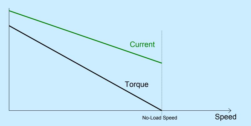
The Torque curve for a PM-DC motor is a straight line descending from the stall torque at zero speed to zero torque at the no-load speed.
