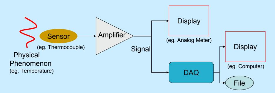
•Some physical phenomenon (such as temperature or strain) is converted into an electrical signal by a sensor.
