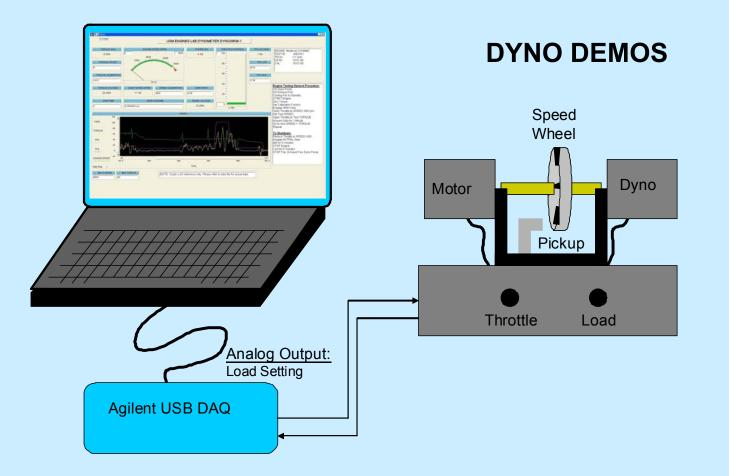
This is an example of an electric motor Dynamometer.
