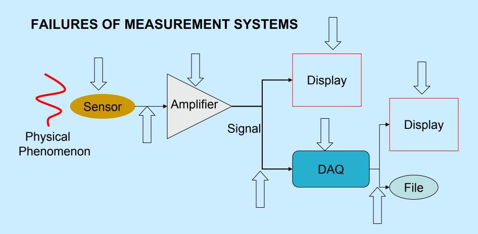
Most failures are noticed only at the "Display" level: either the system is not responding, or responding incorrectly.
