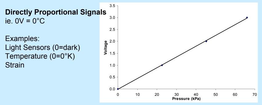
This kind of signal is common when an amplifier has been used which is calibrated to "zero" at 0 units. It is easiest to read as there is no "offset" in the signal.
