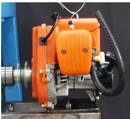
Fig. 1 Carburetor side view of the two-stroke analyzed in this study. Dynamometer coupling is on the left.
