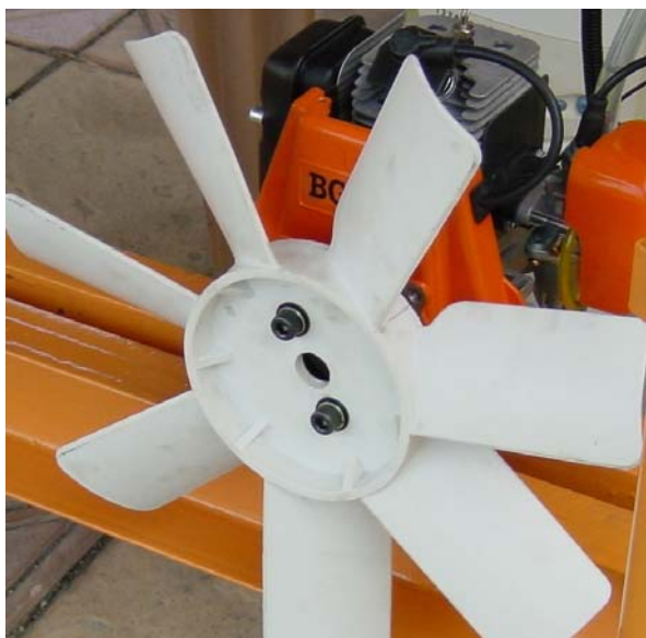
Figure 3 Fan dynamometer coupled to test engine
